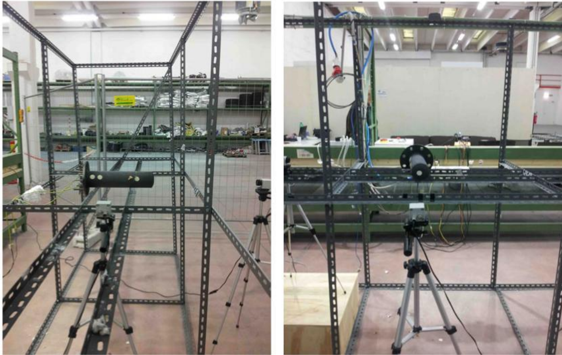
Fig. 12. Two images of the E-Cat HT2. The first displays one of the sides, as framed by one thermal camera, the second displays the breech, framed by the second IR camera. The adhesive “dots” used to evaluate paint emissivity are visible in both images. Note how, in the image on the left, one of the dots is about to fall off due to the heat from the underlying area.
