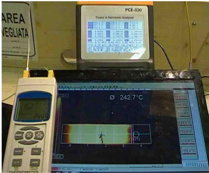
Fig. 13. Dummy measurement set-up. Center: laptop display showing the thermal image of the dummy divided into 5 areas, and the dark shadow of the thermocouple, with probe point located under a dot. Left: thermocouple LCD display, indicating a temperature of 244.5°C. This is relevant to the same area which the IR camera reading of 242.7°C, visible on the laptop display, refers to. The difference is most likely caused by lower thermal exchange between the probe and the environment..
